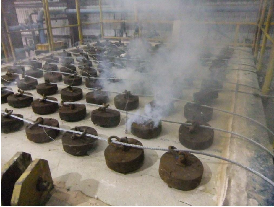
Plate 6 Unexposed face of test construction after approx. 26 minutes from start of test.
