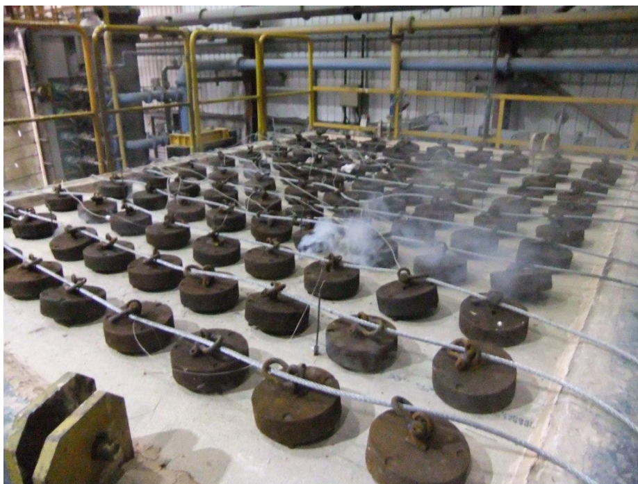
Plate 5 Unexposed face of test construction after approx. 22 minutes from start of test.
