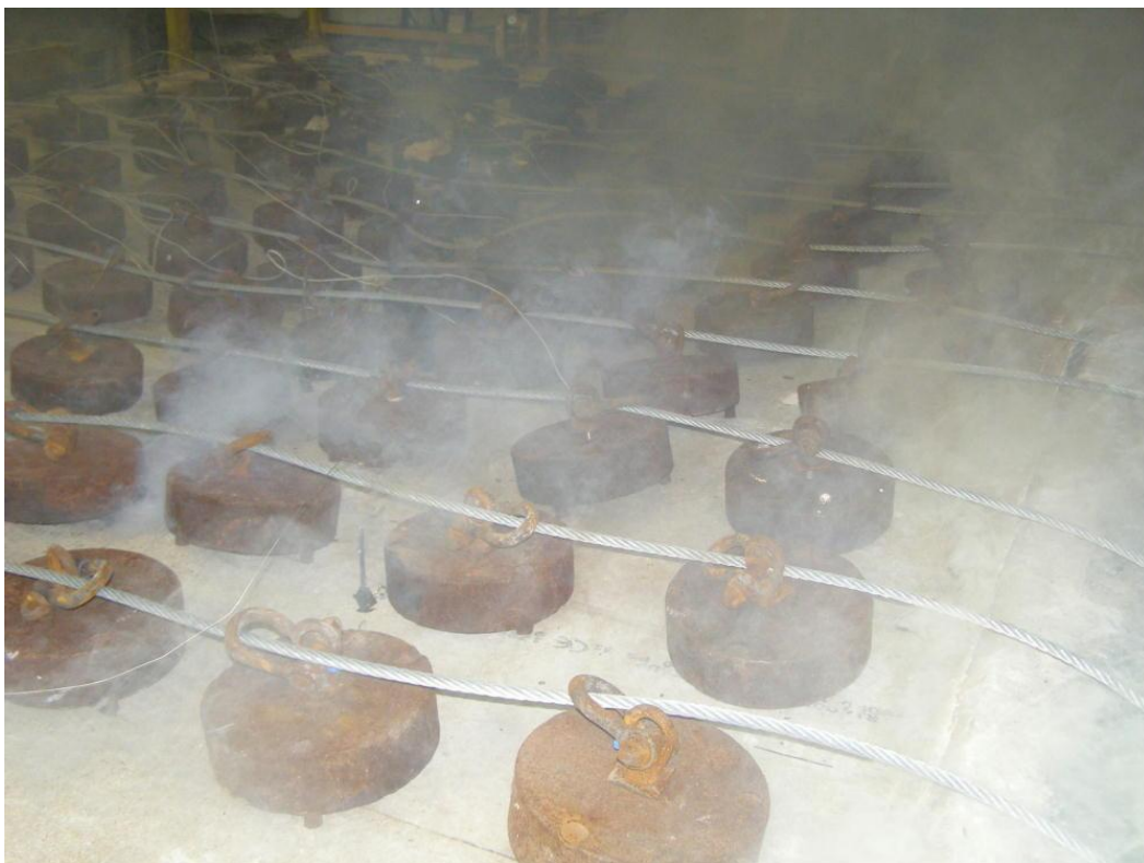
Plate 7 Unexposed face of test construction after approx. 30 min from start of test.
