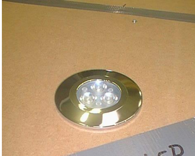
Figure A2. The room face of the Halers H2 down light fitting
